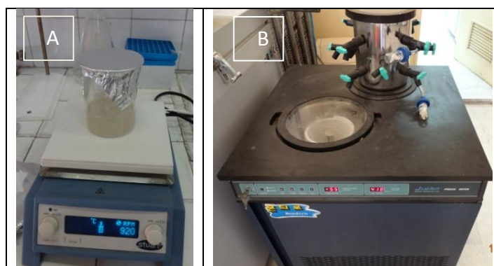
Figure 4. (A): dissolving chitosan powder in acetic acid solution with magnetic stirring. (B): lyophilizing the chitosan with freeze-dryer
