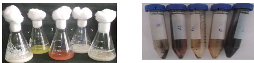
Figure 4 . 1. Reducing \text{Ag}^+ ion to \text{Ag}^0 using fungi as reducing agent Aspergillus fumigatus , 2. Phomopsis Sp, 3. Fusarium oxysporum , 4. Cladosporium, cladosporoides , 5. Colletrotrichum Sp
