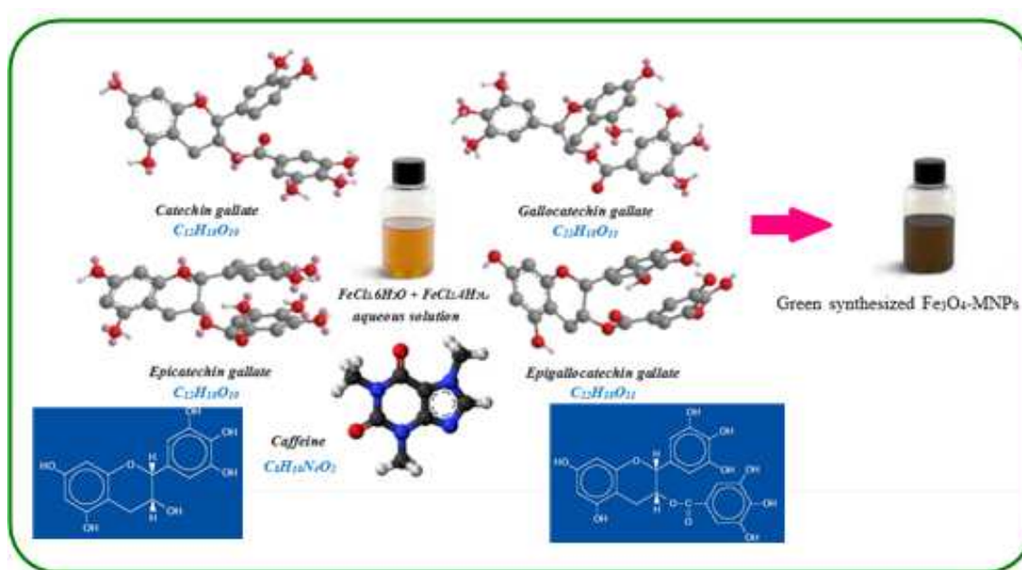
Figure 3. Schematic illustration of synthesized \text{Fe}_3\text{O}_4 -MNPs in White tea( Camelia sinensis ) extract
