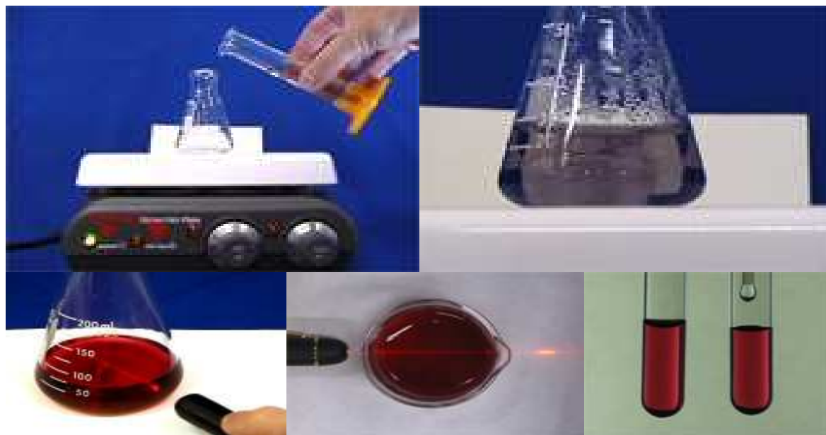
Fig.3 Steps of Gold Nanoparticles Synthesis
