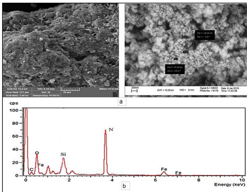
Figure 4: a) FESEM image of poly (ABA-SMA)-APTES-Fe<sub>3</sub>O<sub>4</sub>MNC b) EDX spectrum of Modified (SMA)-APTES-Fe<sub>3</sub>O<sub>4</sub> nanoparticles
