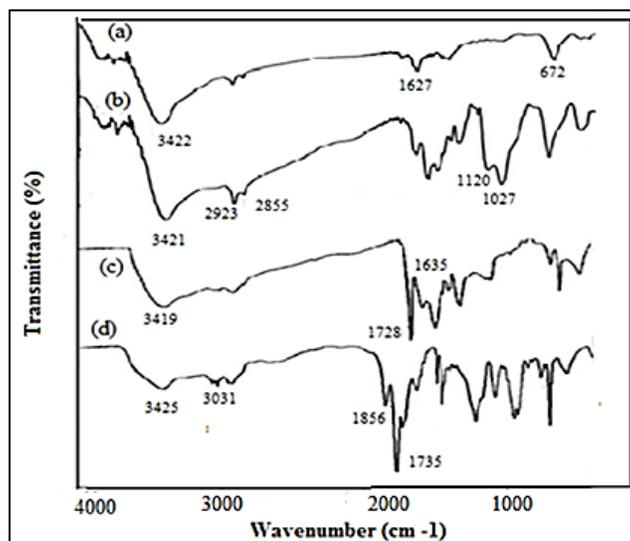
Figure 2: FT-IR spectrum, a)  $\text{Fe}_3\text{O}_4$  b) APTES (3-aminopropyltriethoxysilane), c) APTES/SMA, d) SMA
