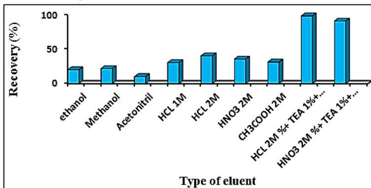
Figure 8: Effect of eluent type and concentration on the recovery of 10 µg L<sup>-1</sup> atenolol. Experimental conditions: pH; 7, amount of sorbent; 150 mg, sample volume; 50 mL)
