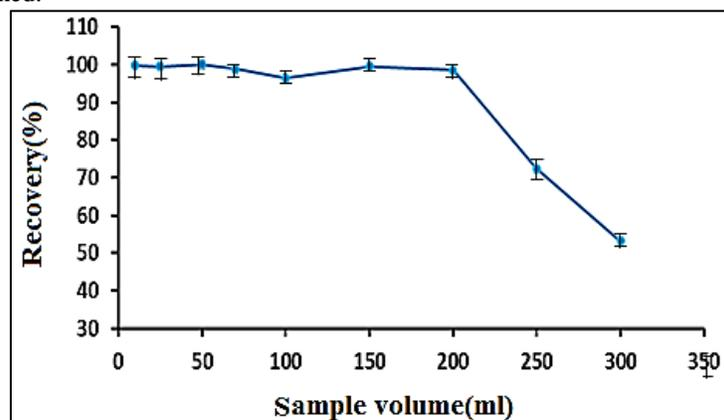
Figure 9: Evaluation of the extraction efficiency of atenolol by using the different sample volumes and constant amount of poly (ABA-SMA)-APTES-Fe<sub>3</sub>O<sub>4</sub>MNC as sorbent, utilized conditions: atenolol, 10µg L<sup>-1</sup>; phosphate buffer (pH 7.0); MNC, 150 mg; eluent volume 2 mL of (HCl 2M+ TEA 1%+ TFA 1%); centrifugation time, 5 min
