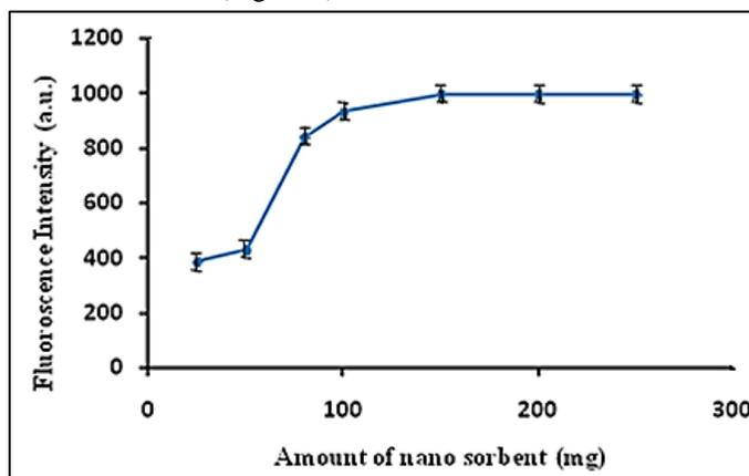
Figure 7: Effect amount of nano sorbent on the extraction efficiency of atenolol utilized conditions: atenolol  $10 \mu\text{g L}^{-1}$ ; (pH 7.0); 3 mL of (HCl 2M+ TEA 1%+ TFA 1%) as eluent; centrifugation time, 20 min
