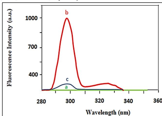
Figure 5: Fluorescence spectrum of the (a) blank, (b) atenolol in the presence (c) atenolol in the absence of the sorbent
