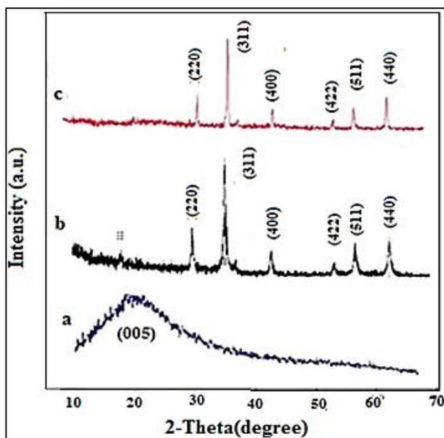
Figure 3: XRD pattern of (a) SMA (b) poly (ABA-SMA)@APTES- $\text{Fe}_3\text{O}_4$  MNC (c)  $\text{Fe}_3\text{O}_4$  MNC nanohybride, respectively
