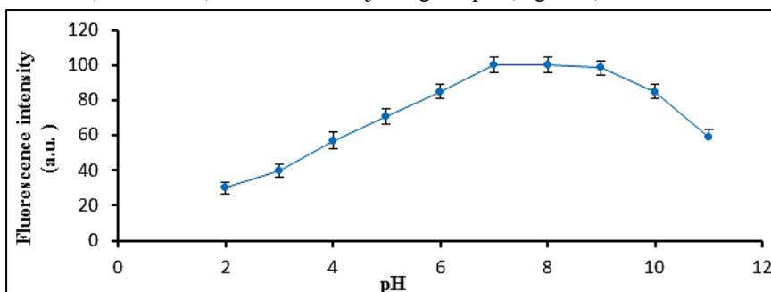
Figure 6: Effect of pH on the extraction efficiency of atenolol utilized conditions: atenolol  $10 \mu\text{g L}^{-1}$ ; poly(ABA-SMA)-APTES- $\text{Fe}_3\text{O}_4\text{MNC}$  (magnetic nano sorbent), 200 mg; 3 mL of (HCl 2M+ TEA 1%+ TFA 1%) as eluent; centrifugation time, 20 min
