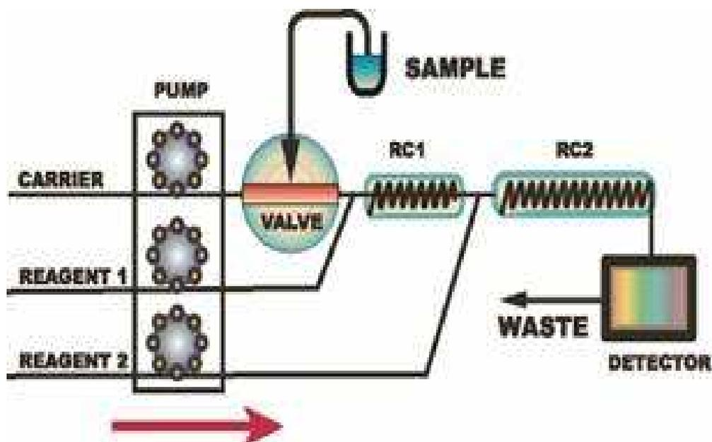
**Fig 3: Flow injection analyzer**
