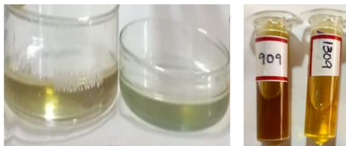
Figure 5: After direct trans-esterification process, the converted FAMES were labeled and stored in a separate fresh eppendorf at -20°C to avoid degradation until GC-FID analysis
