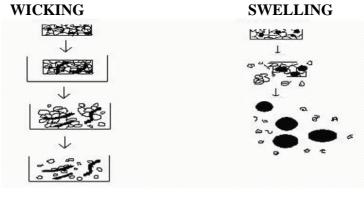
Water is pulled by disintegrant And reduced the physical Bonding force between particles
