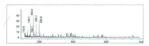
Figure 17. MS Report for the Separated Fraction1 (Time 0.493:0.772)
