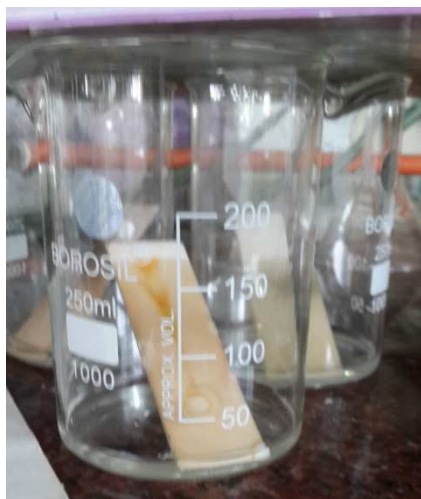
Fig.3 TLC plate inside developing chamber
