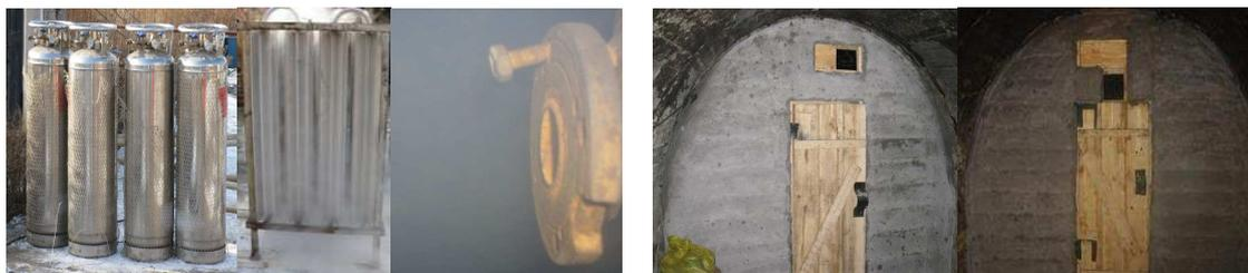
Fig. 2 Inert gas injection system and bulkheads
