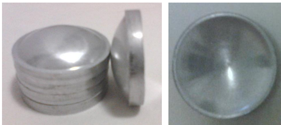
Figure 1. The shaped charge liner by mould pressing
