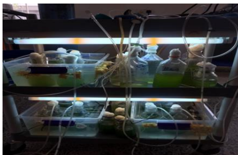
Figure 3: Experimental setup of Chlorella vulgaris culture under aeration culture
