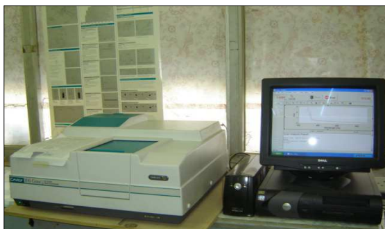
Figure (2): UV-visible –spectrophotometer (EL 04113001, varian, U.S.A.)
