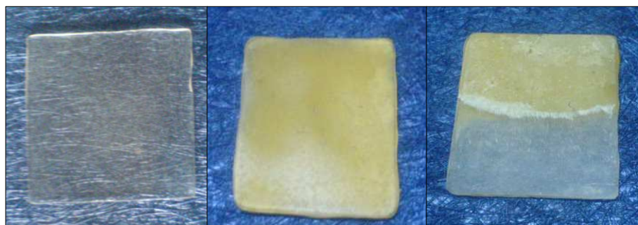
Fig. (5): Adhesive failure Fig. (6): Cohesive failure Fig. (7): Mixed failure
