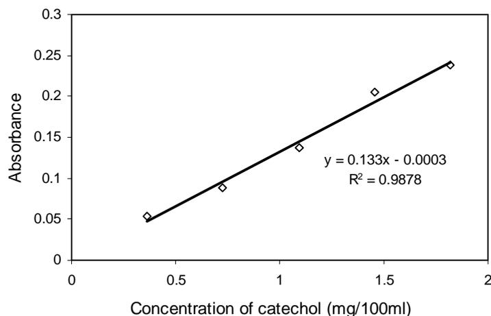
**Fig.2:** Calibration plot for flavonoid determination at 415 nm
