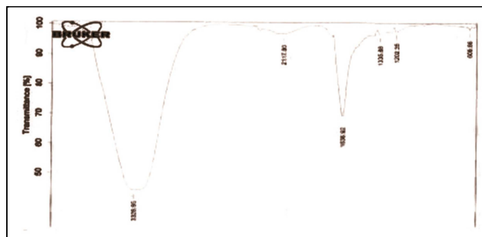
Figure 2: FTIR spectroscopy analysis of AgNPs synthesized using A. vasica
