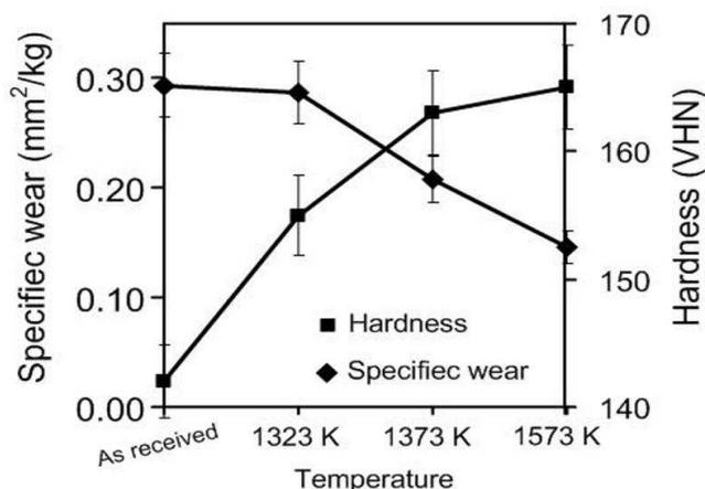
Fig. 5. Specific wear and hardness at the surface
