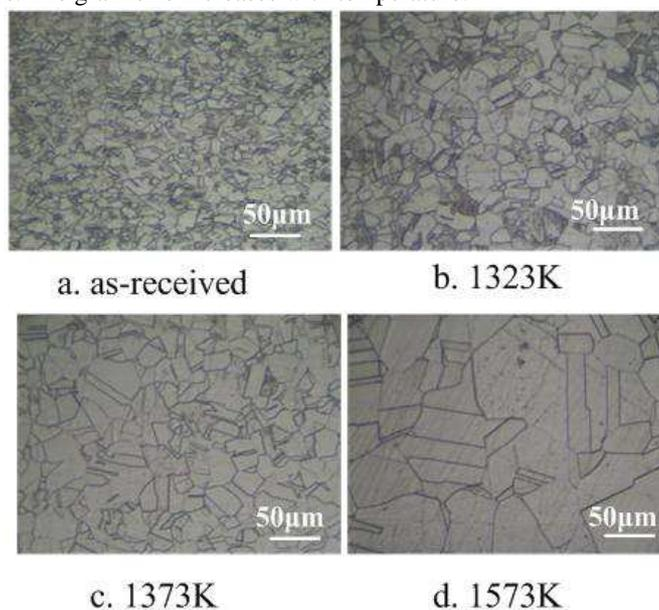
Fig. 2. Microstructure of specimens 316LVM
