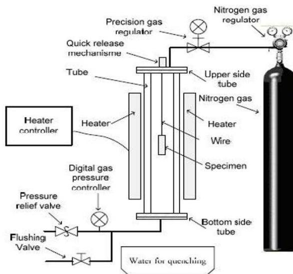
Fig. 1. Schematic of modified vertical furnace
