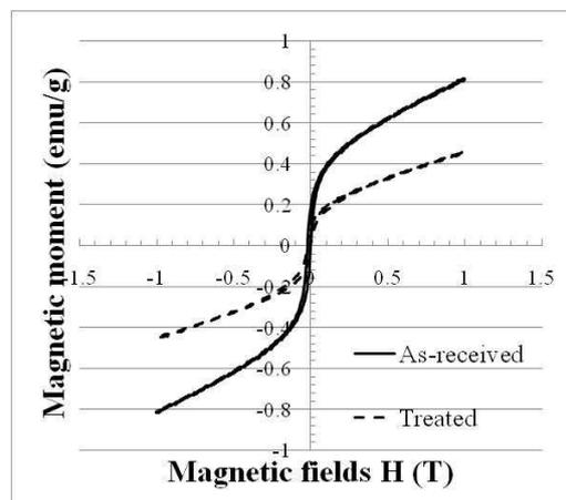
Fig. 7. Magnetization curve of specimens
