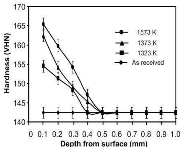
Fig. 4. Hardness distribution of as received and treated specimens
