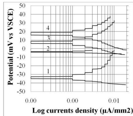
Fig. 6. Polarization curve. 1. as received, 2. 1323 K, 3. 1373 K & 4. 1573 K
