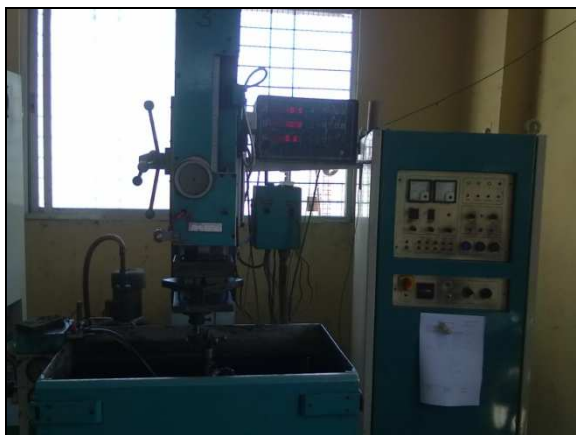
Figure 1 EDM experimental set up
