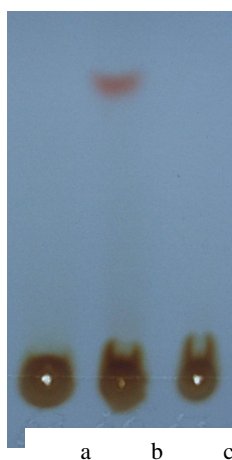
Fig. 1 Thin layer chromatography (TLC) of (a) yeast fermentation broth, (b) chloroform extract from the fermentation broth of mutant strain N6076 and (c) chloroform extract from the fermentation broth of original yeast strain
