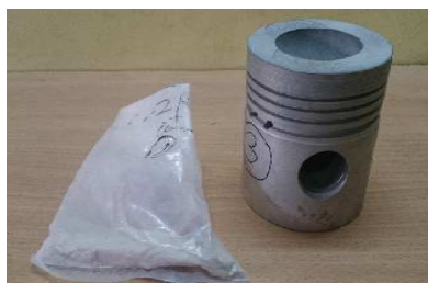
Fig.5 \text{ZrO}_2 . \text{CeO}_2 Coated Piston
