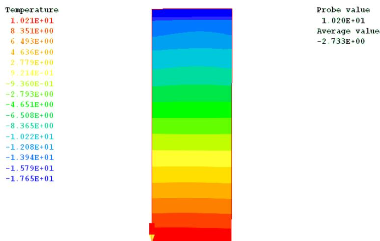
Fig.2 The temperature field of refrigerated warehouse floor that ventilation system isn't circulating
