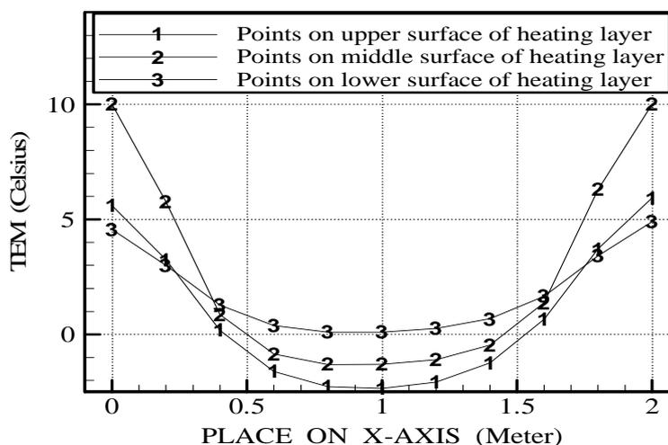
Fig.6 The temperature distribution curves of points at Z=1m on upper, middle and lower surface for heating layer with 2.0m tube spacing
