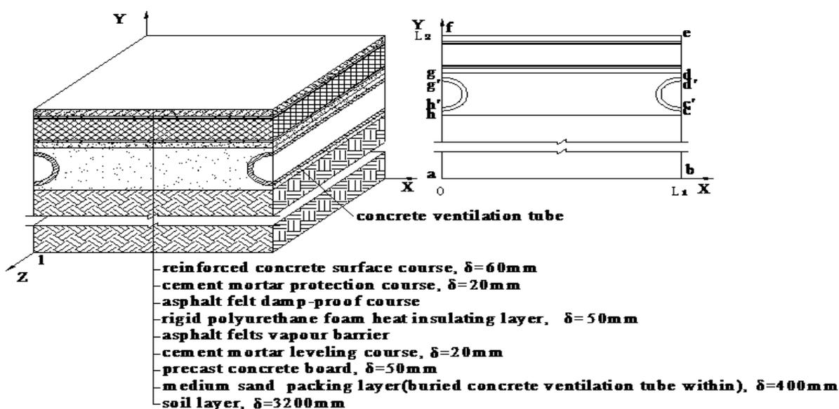
Fig.1 The calculating unit of heat transfer model for refrigerated warehouse floor
