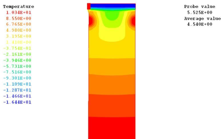
Fig.3 The temperature field of refrigerated warehouse floor that ventilation system is circulating with 1.5m tube spacing
