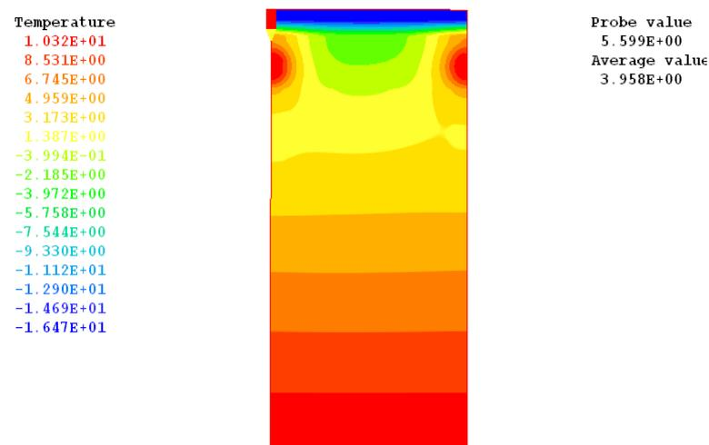
Fig.4 The temperature field of refrigerated warehouse floor that ventilation system is circulating with 2.0m tube spacing
