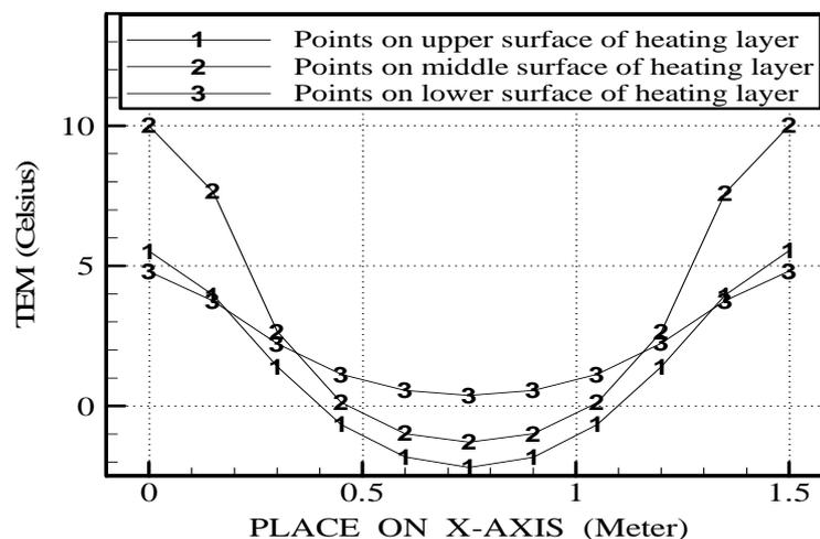
Fig.5 The temperature distribution curves of points at Z=1m on upper, middle and lower surface for heating layer with 1.5m tube spacing
