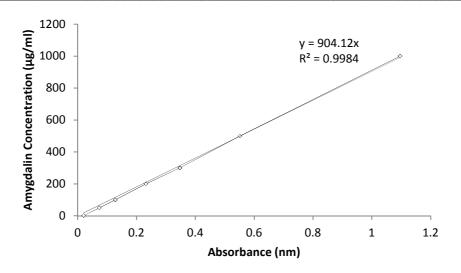
Figure 3: Amygdalin calibration curve
