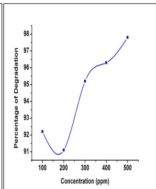
Fig.10. Effect of initial concentration on phenol degradation rate
