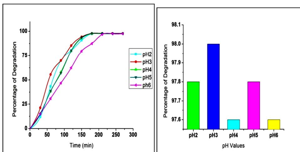
Fig.3. Variation of phenol degradation with time at different pH values
