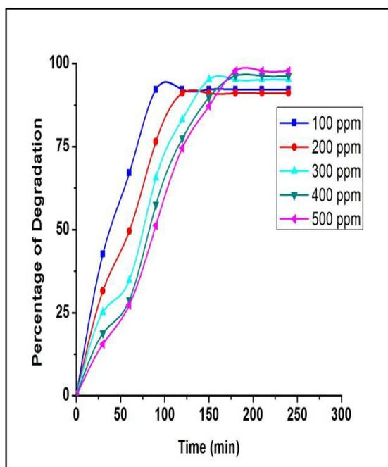
Fig.9. Variation of phenol degradation with time at different initial concentrations
