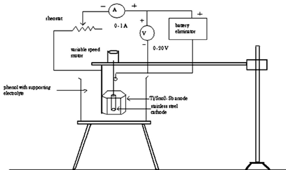
Fig.2. Circuit diagram for phenol electrolysis for electrochemical method
