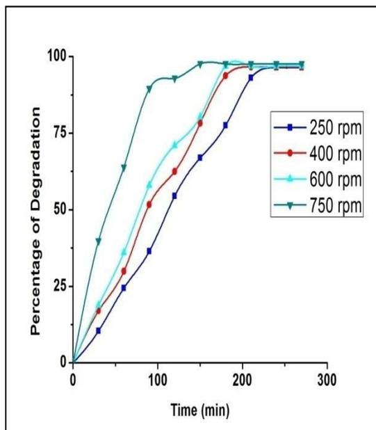
Fig.11. Variation of phenol degradation time at different cathode speeds
