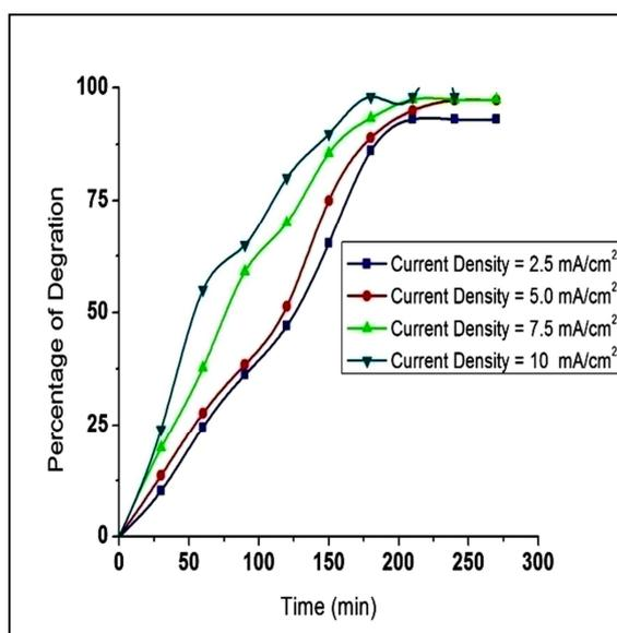
Fig.5. Variation of phenol degradation with time at different current densities
