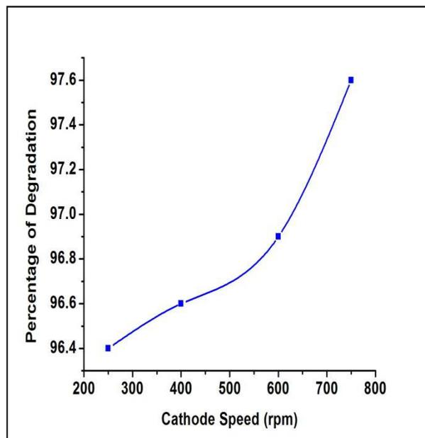
Fig.12. Effect of cathode speed on phenol degradation rate
