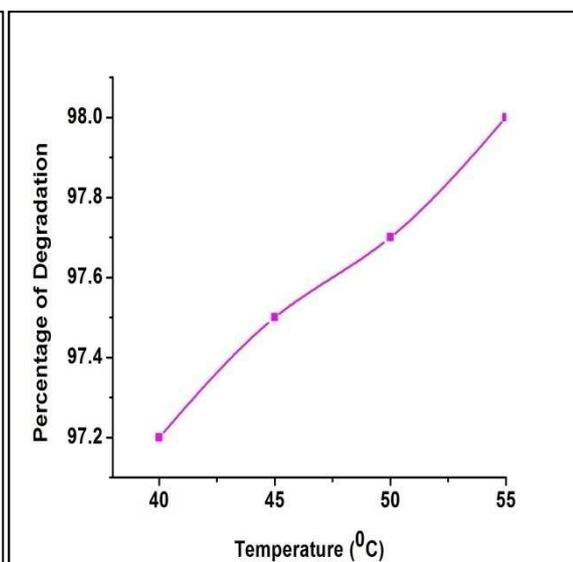
Fig.8. Effect of temperature of phenol degradation rate
