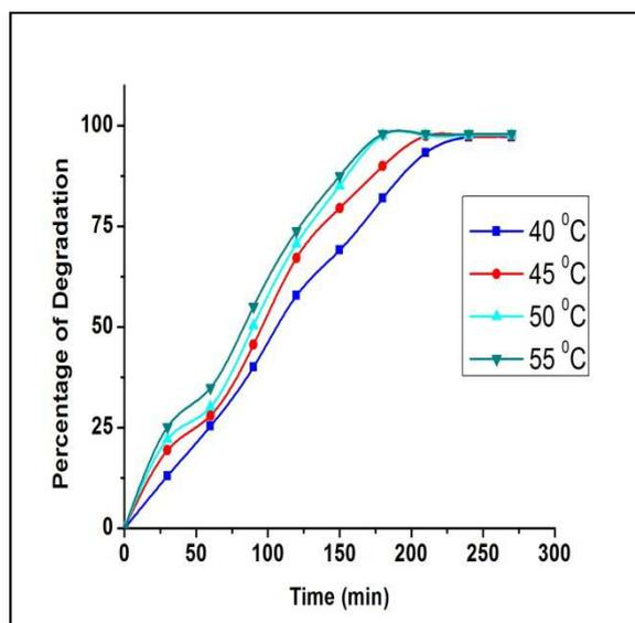
Fig.7. Variation of phenol degradation with time at different electrolysis temperatures
