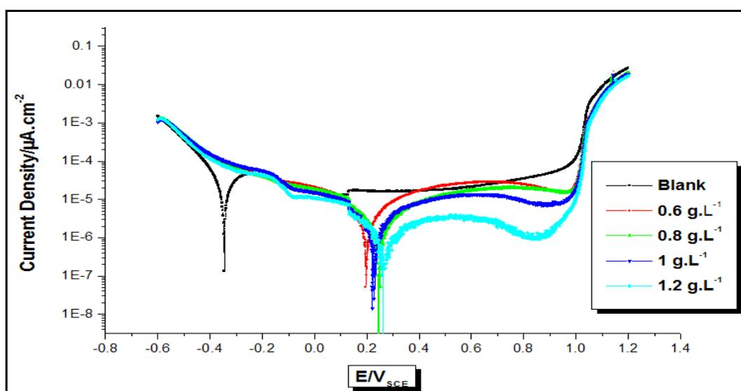
Figure 4. Polarization curves of stainless steel in concentrated H<sub>3</sub>PO<sub>4</sub> at different concentrations of organic oil [L]
