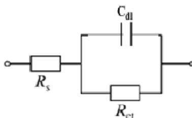
Figure 6. Equivalent circuit model for the corrosion for welded material in 5.5M H<sub>3</sub>PO<sub>4</sub> at 298 K
