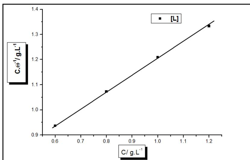
Figure 8: Langmuir isotherm adsorption model on the stainless steel surface of [L] in 5.5 M  $\text{H}_3\text{PO}_4$
