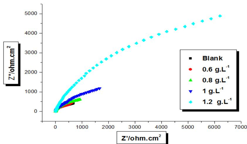
**Figure5. Nyquist diagrams for welded material in 5.5M H<sub>3</sub>PO<sub>4</sub> containing different concentrations of organic oil [L]**
