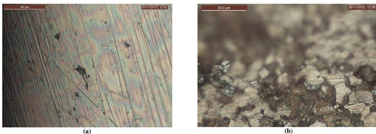
Figure 7 : Examination by electron microscopy of the surface of the alloy welded phosphoric medium
