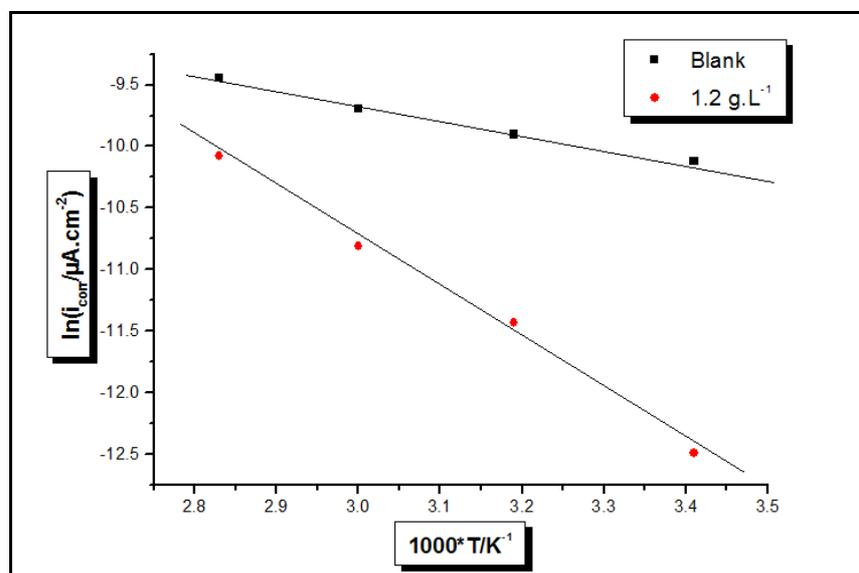
**Figure 9: Arrhenius straight lines calculated from corrosion rate of stainless steel in 5.5M H<sub>3</sub>PO<sub>4</sub> and 5.5M H<sub>3</sub>PO<sub>4</sub> + 1.2g.L<sup>-1</sup> [L]**
