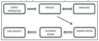
Figure 1: Freeze drying process
