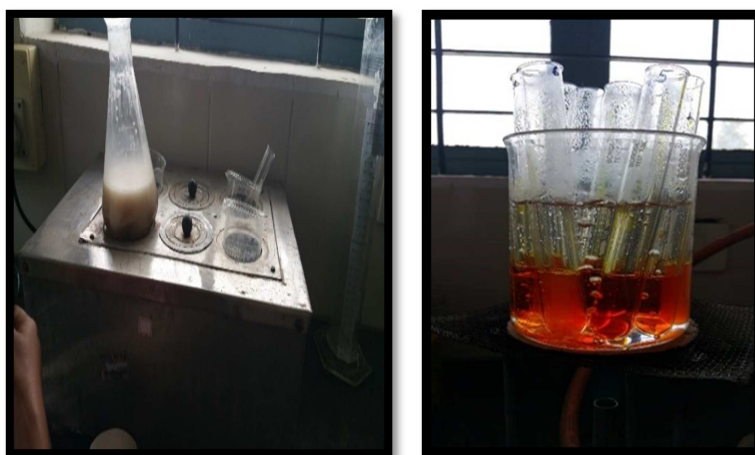
Figure 1: TKP solution kept in water bath at 80 o C, DNSA test of the sample solution
