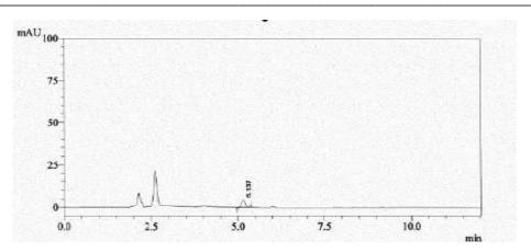
Fig.3. Representative Chromatogram of kresoxim methyl test item in basic water - day 0
