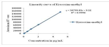
Fig.4. Representative Calibration curve of kresoxim methyl standard
