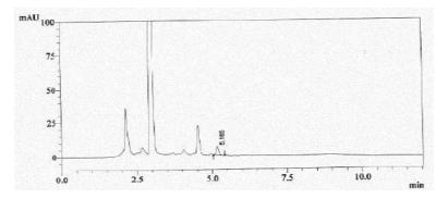
Fig.2. Representative Chromatogram of kresoxim methyl test item in neutral water - day 0
