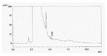
Fig.1. Representative chromatogram of kresoxim methyl test item in acidic water - day 0
