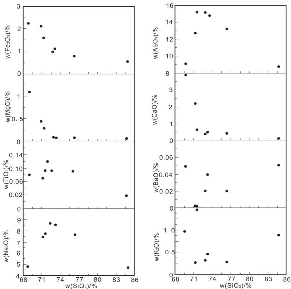
Figure 7 Harker Diagram for Major Oxides of Sample Special Lithological Layers at Ping Chau Formation
