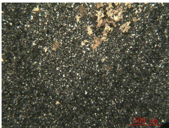
Figure 6 Rhyolite Crystal Pyroclasts Vitroclastic Tuff (Cross-polarized Light)
