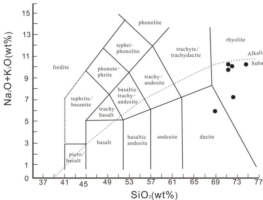
Figure 8 TAS Analysis Diagram for Sample Special Lithological Layers at Ping Chau Formation (Classification Based on Middlemost,1994; Boundaries Based on Irvine & Baragar,1971)
