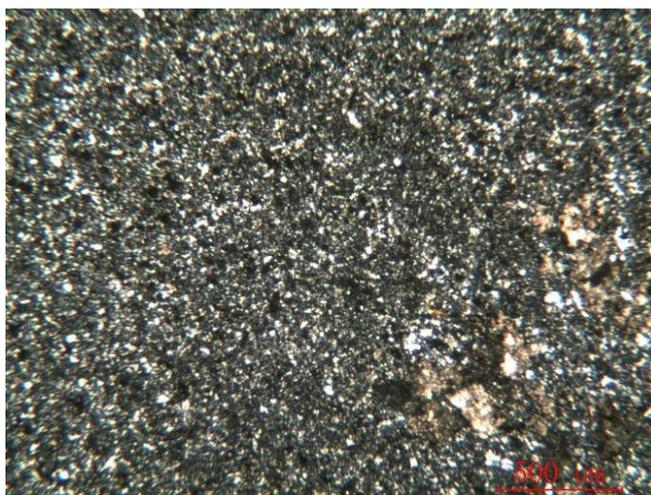
**Figure 3** Microstructure Picture of Rhyolite Vitroclastic Tuff (Cross-polarized Light)
