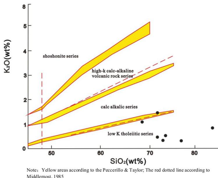
**Figure 10 K<sub>2</sub>O-SiO<sub>2</sub> Diagram for Sample Special Lithological Layers at Ping Chau Formation**
