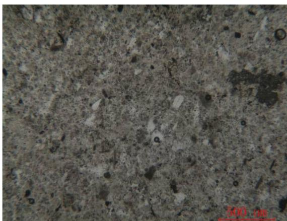
Figure 2 Microstructure Picture of Dacite (Cross-polarized Light)
