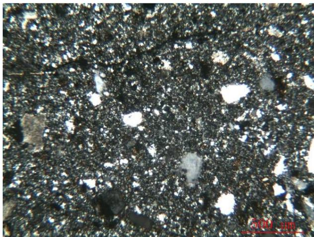
Figure 5 Microstructure Picture of Rhyolite Vitroclastic Tuff (Cross-polarized Light)
