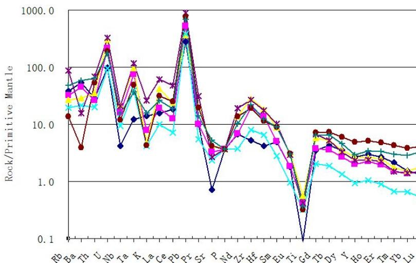
Figure 12 Standardized Spider Diagram for Microelements in Primitive Mantle of Sample special lithological layers at Ping Chau Formation (Based on Standardized Data of Sun & Mc Donough,1989)
