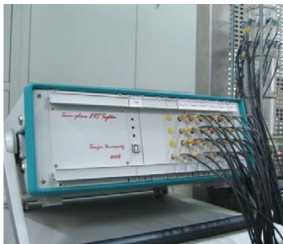
Fig. 3: The digital dual-plane ERT system
