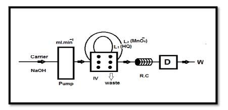
Figure(10): Flowgram of the whole manifold with double loop -6- three way valve (IV; injection valve, RC; reaction coil, D; detector, W; waste)
