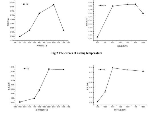
The curves of ashing temperature are shown in Fig 2 and atomization temperature are shown in Fig3.
