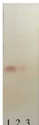
Figure 2: TLC of samples prepared from modified milk. (1) standard histamine; (2) extract to detect histamine; (3) negative control
