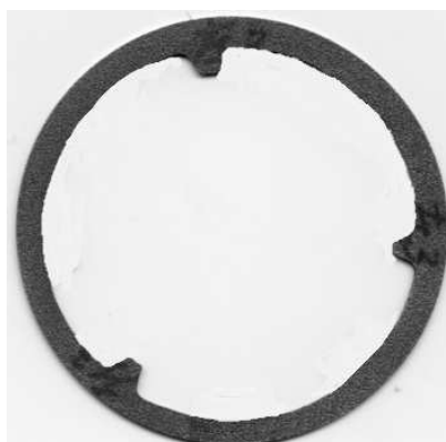
Fig.12: The sample piece of ECM for chamber body inner cavity
