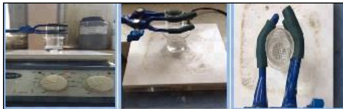
Figure 2: Modified disintegration test apparatus used to determine the disintegration time of the prepared ODTs of Zolmitriptan
