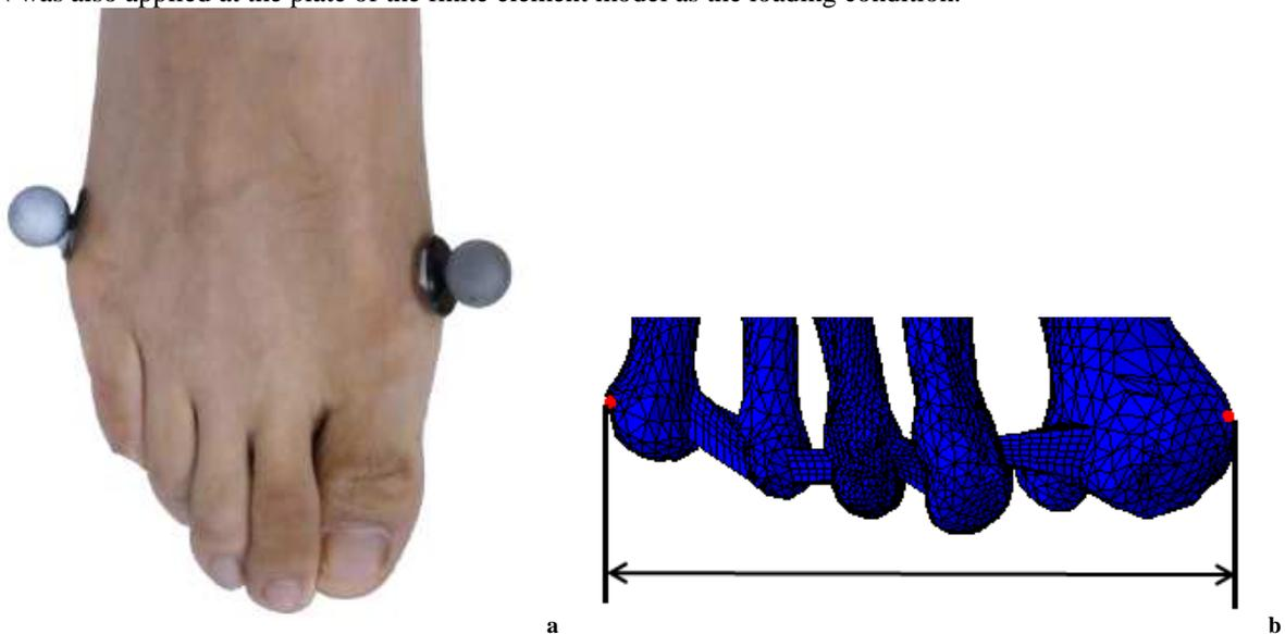
**Fig.2** The experimental measurement (a) and simulation prediction (b) methods of the forefoot transverse deformation
