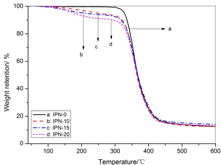
Figure 4: TGA thermograms of (a) IPN-0, (b) IPN-10, (c) IPN-15 and (d) IPN-20
