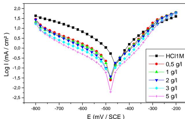
Figure 1. Potentiodynamic polarisation curves of mild steel in hydrochloric acid solution with and without inhibitor at different percentages of juice fruit OFI
