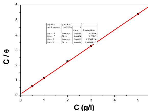
Figure 3. Langmuir isotherm adsorption model of OFI on the steel surface in 1M HCl
