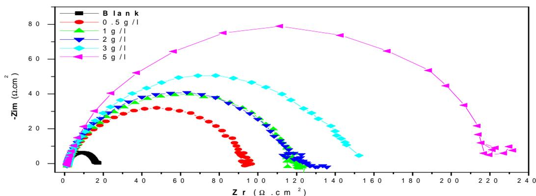
Figure 2. Impedance plot of mild steel obtained in 1M HCl in the absence and presence of various concentrations of OFI
