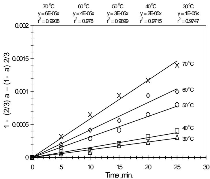
**Fig. 6: Leaching kinetics of calcium from phosphogypsum by HNO<sub>3</sub>-NPE**
