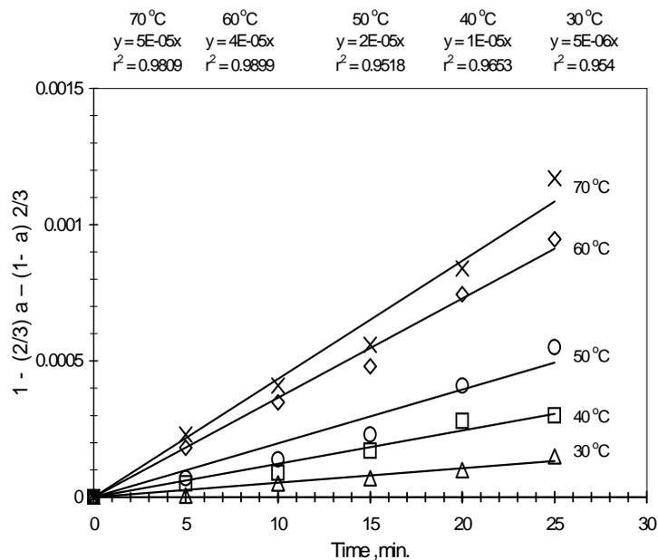
Fig. 7: Leaching kinetics of calcium from phosphogypsum by HCl-NPE
