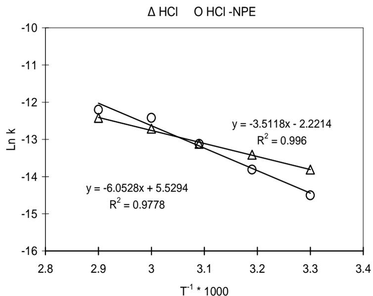
Fig. 9: Activation energy of calcium leaching from phosphogypsum by HCl and HCl-NPE
