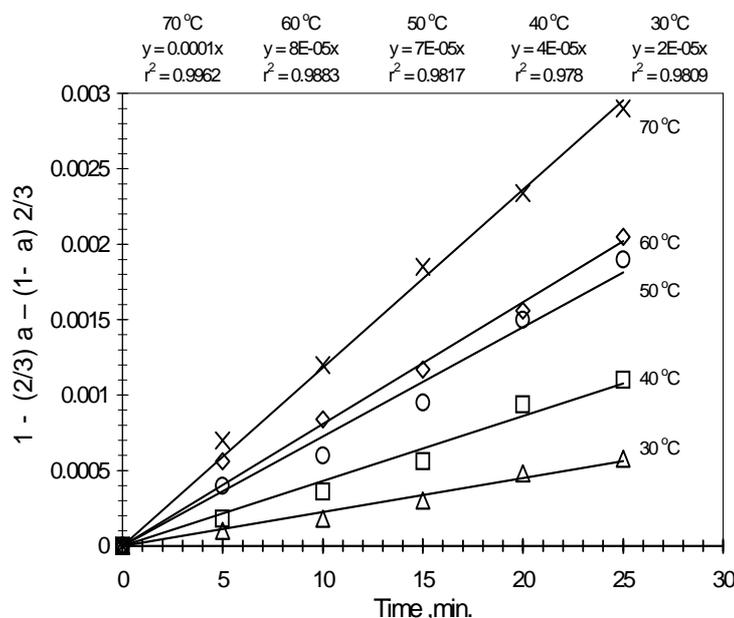
Fig. 4: Leaching kinetics of calcium from phosphogypsum by  $\text{HNO}_3$
