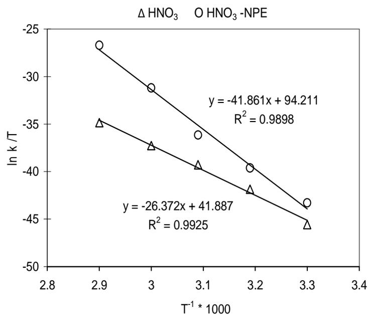
Fig. 10: Enthalpy and entropy of calcium leaching from phosphogypsum by HNO<sub>3</sub> and HNO<sub>3</sub>-NPE
