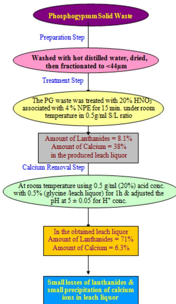
Fig.12. Flow Sheet of calcium dissolution controlling process
