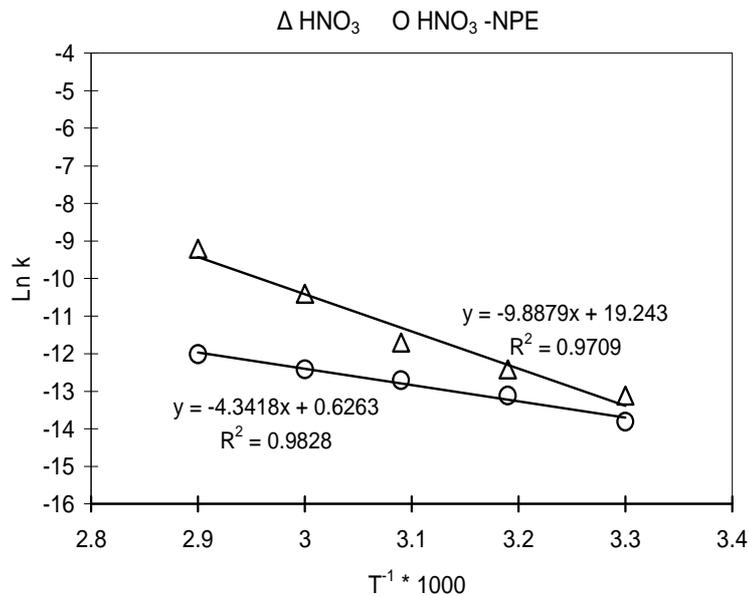
Fig. 8: Activation energy of calcium leaching from phosphogypsum by HNO<sub>3</sub> and HNO<sub>3</sub>-NPE
