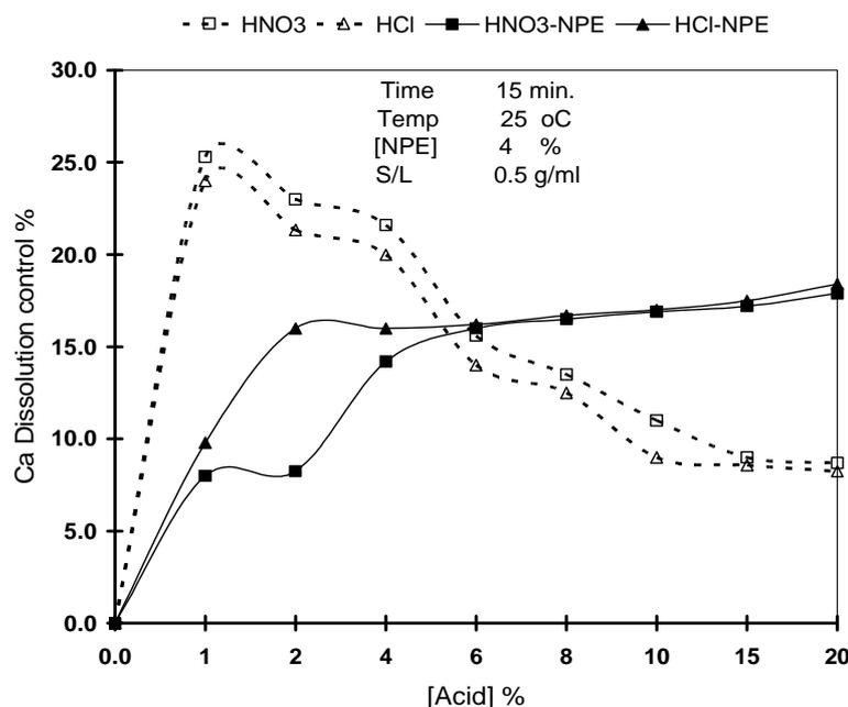
Fig. 1: Effect of acid concentration on the calcium dissolution control %
