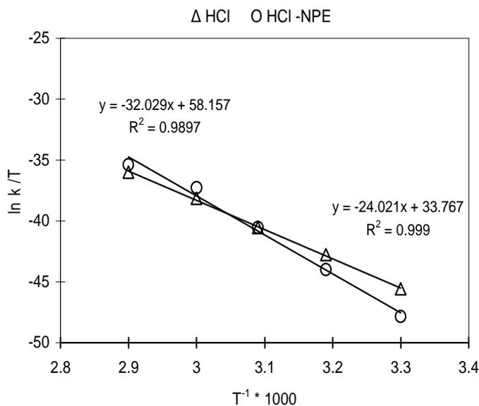
Fig. 11: Enthalpy and entropy of calcium leaching from phosphogypsum by HCl and HCl-NPE
