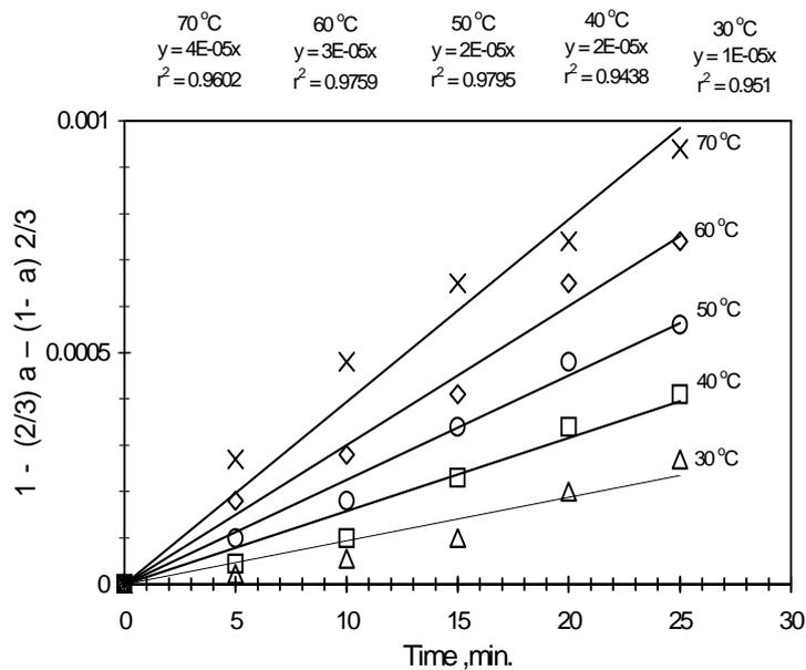
**Fig. 5: Leaching kinetics of calcium from phosphogypsum by HCl**
