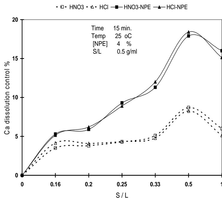
Fig. 2: Effect of solid to liquid (S/L), g/ml on the calcium dissolution control %
