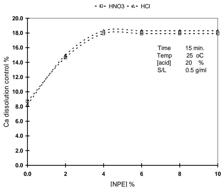
Fig. 3: Effect of NPE concentration on the calcium dissolution control %
