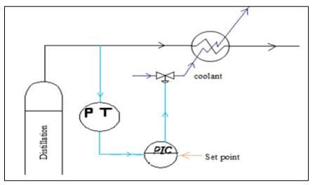
Figure 2: Process control diagram for fractionator overhead pressure
