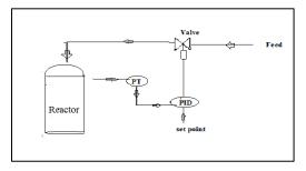
Figure 1: Process control diagram for soaker overhead pressure
