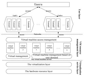
Fig. 1 The model of calculating resource pool
