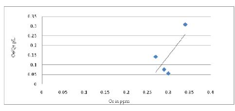
Fig.6 Langmiur isotherm for inactivated coconut husk
