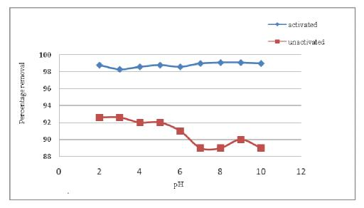
Fig.3 Effect of ph by activated and inactivated coconut husk
