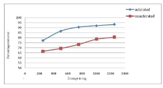
Fig.4 Effect of adsorbent dosage by activated and inactivated coconut husk
