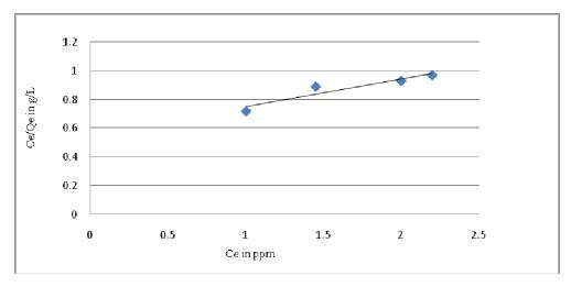
Fig.5 Langmiur isotherm for activated coconut husk
