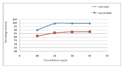
Fig.2 Effect of initial metal ion concentration by activated and inactivated coconut husk
