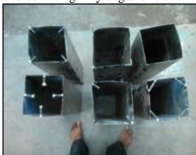
Figure 2: Steel tube mould with stiffeners
