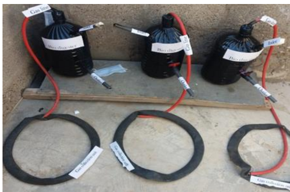
Figure 2. Set up of the digester and operational digester
