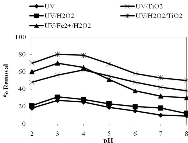
**Figure 3: Effect of pH on degradation of H-acid**
