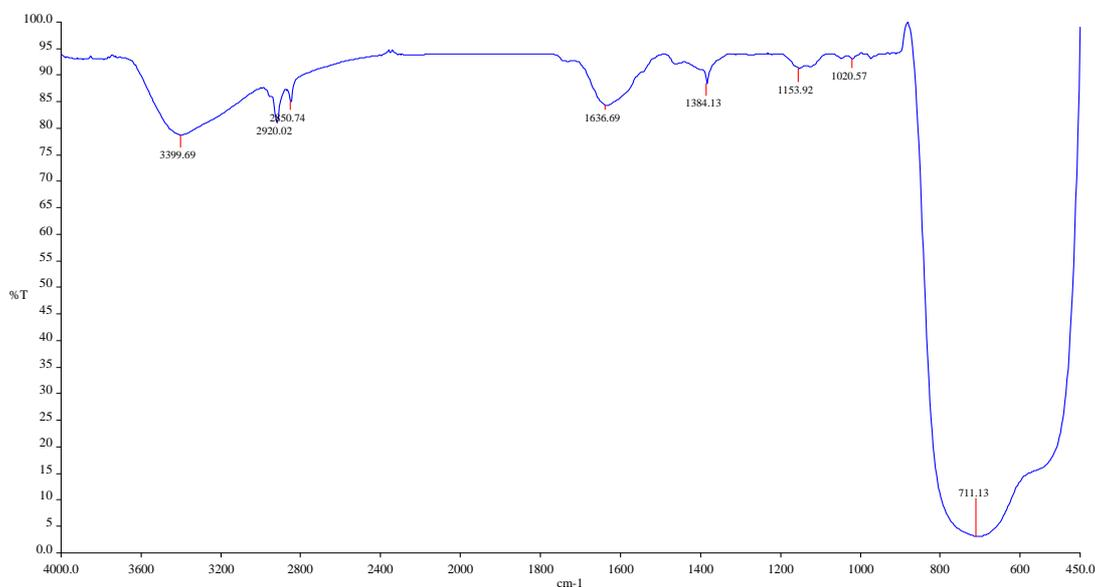
**Figure 6: FTIR Spectrum of  $\text{TiO}_2$**
