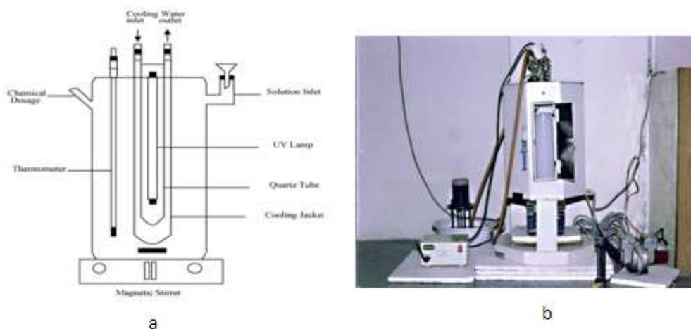
**Figure 1. (a) Schematic representation of photo reactor (b) Photographic view of 16W UV Photo Reactor**
