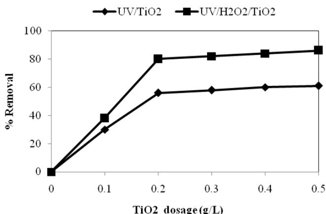
Figure 5: Effect of  $\text{TiO}_2$  dosage on degradation of H-acid
