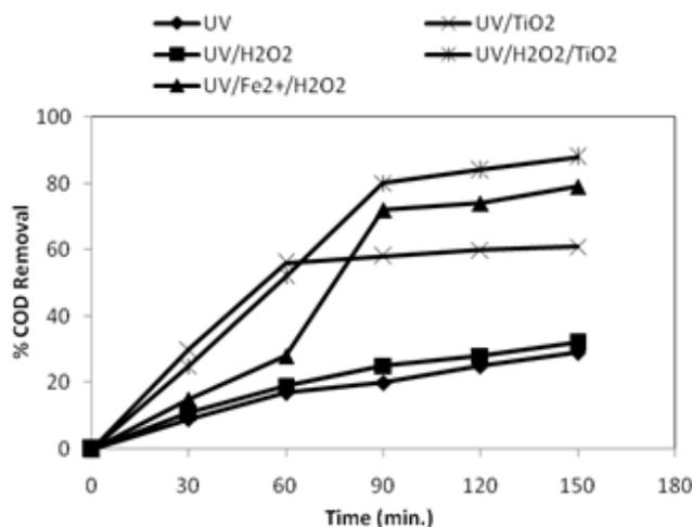
Figure 9: COD removal on the degradation of H-acid
