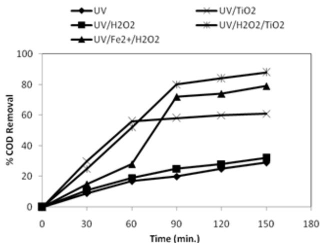
Figure 9: COD removal on the degradation of H-acid
