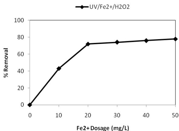
**Figure 8: Effect of  $\text{Fe}^{2+}$  dosage on degradation of H-acid**
