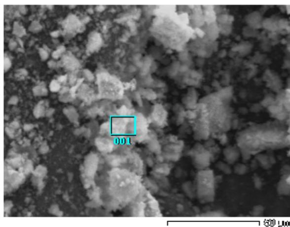
**Figure 7: SEM analysis of  $\text{TiO}_2$**
