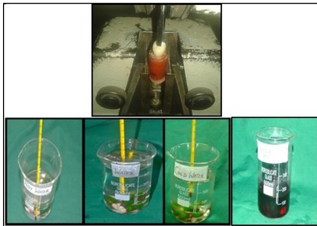
Figure 4: Mechanical loading, thermocycling of samples and immersion in in 0.5% aqueous solution of basic fuschin
