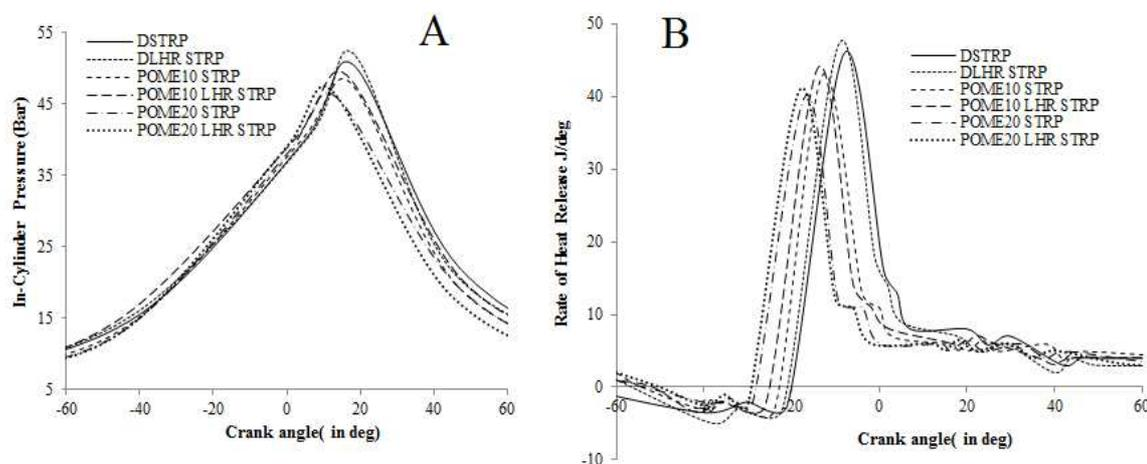
Figure 4. Variation of In-cylinder pressure and Rate of Heat release with Crank angle
