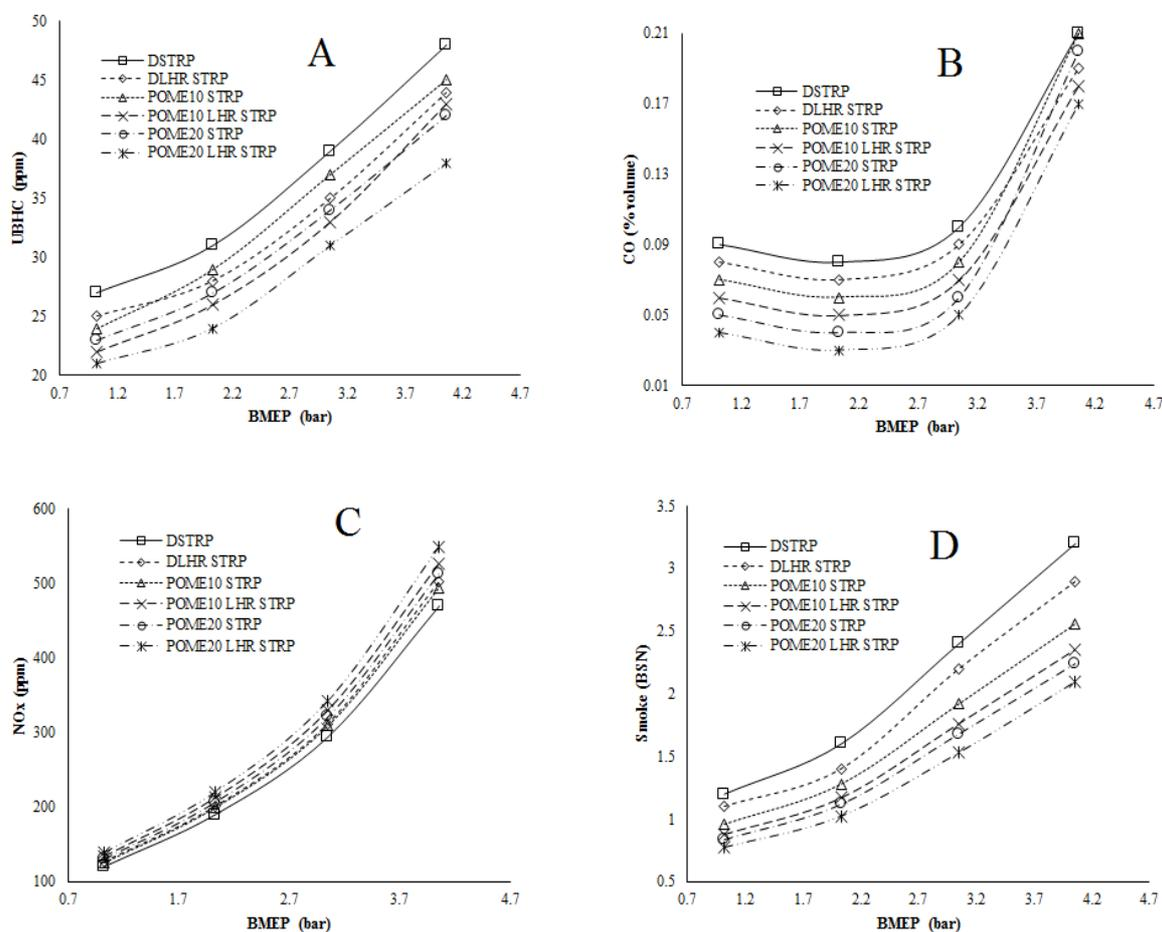
Figure 6. Variation of UBHC (A), CO (B), NO<sub>x</sub> (C) and Smoke (D) with BMEP
