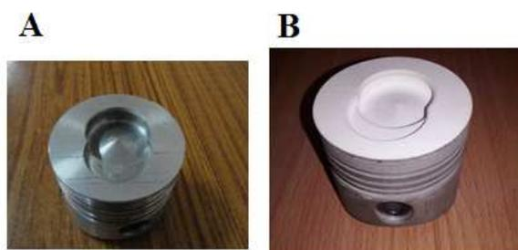
Figure 2. Pictorial view of the STRP without Alumina coating (A) & with Alumina Coating (B)
