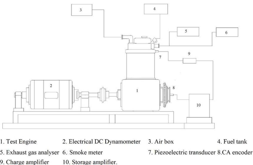
Figure 3. Schematic layout of the Experimental setup
