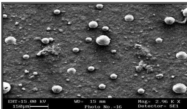
Figure 1: SEM photograph of clarithromycin microspheres
