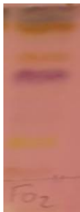
Figure 2. Chromatogram of the chloroform/Ethanol extract (50% v/v) Migration solvent: Hexane/Ethyl acetate (70/30, v / v). Developer: Sulfuric Anisaldehyde
