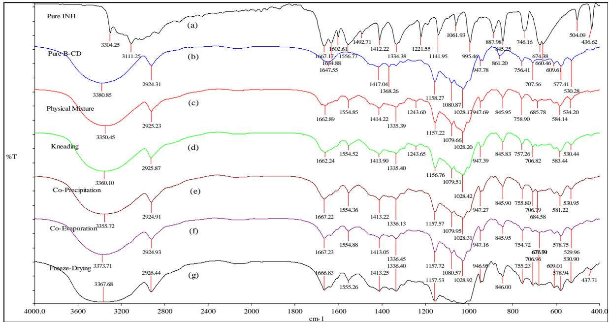
Figure 5: FTIR spectra for isoniazid (a),  $\beta$ -cyclodextrin (b), physical mixture complex (c), kneading complex (d), Co-precipitation complex (e), Co-evaporation complex (f), and freeze-drying complex (g) from 400-4000  $\text{cm}^{-1}$
