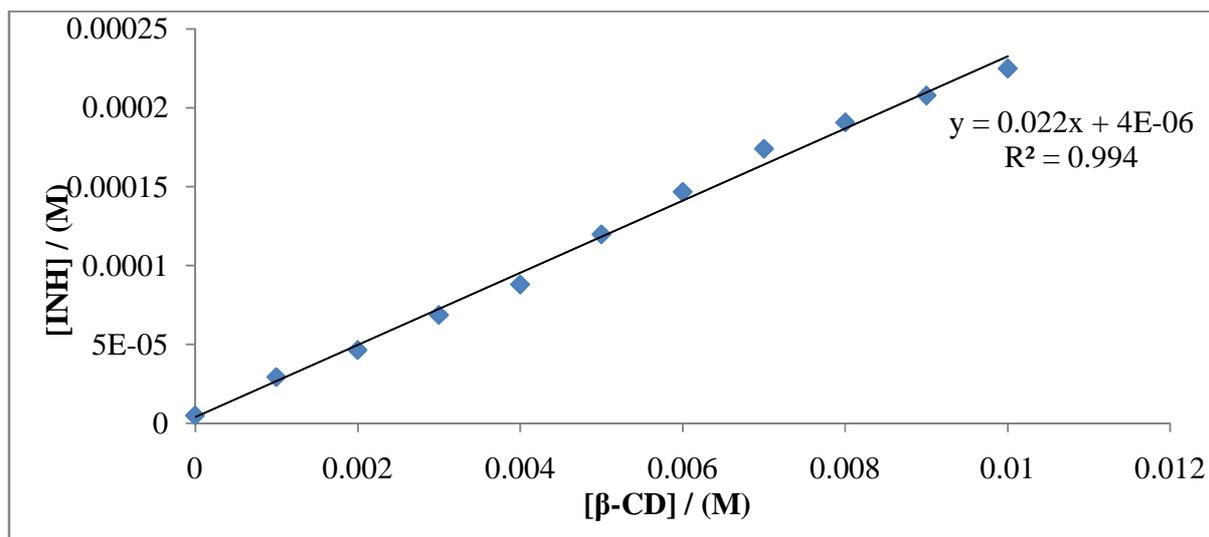
Figure 3: Phase solubility studies profile of isoniazid/ $\beta$ -cyclodextrin complex at  $25^\circ\text{C}$
