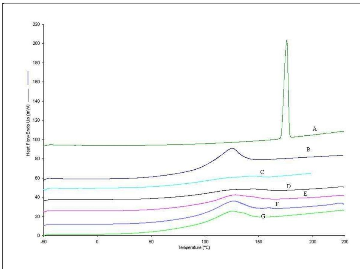
Figure 7: DSC thermogram for isoniazid (A),  $\beta$ -cyclodextrin (B), physical mixture (C), kneading (D), co-precipitation (E), co-evaporation (F) and freeze-drying (G) system
