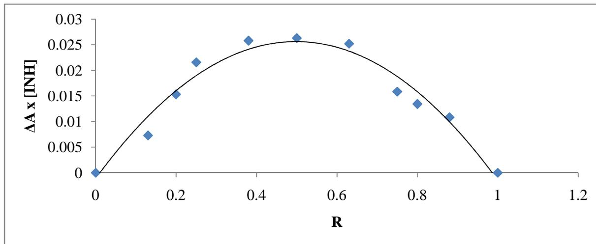
Figure 4: Continuous variation method (Job's plot) for isoniazid/ $\beta$ -cyclodextrin system from absorbance measurements
