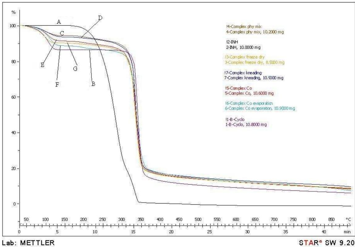
**Figure 6:** TGA thermogram for isoniazid (A),  $\beta$ -cyclodextrin (B), physical mixture (C), kneading (D), co-precipitation (E), co-evaporation (F) and freeze-drying (G) system
