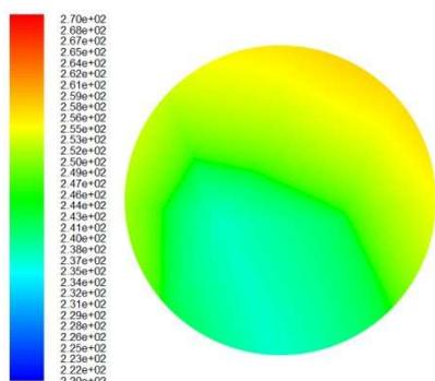
Figure 10. The contour of turbulent intensity in MIJSN
