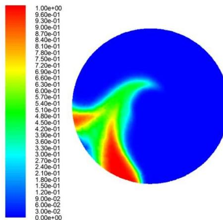
Figure 5. The contour of  $\text{CH}_2\text{Cl}_2$  volume fraction at cross section A-A of jet-swirl nozzle
