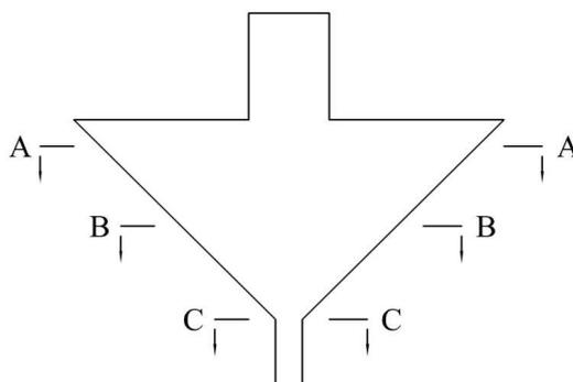
Figure 3. The schematic of cross sections for expressing  $\text{CH}_2\text{Cl}_2$  volume fraction in the mixture
