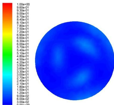
Figure 6. The contour of CH<sub>2</sub>Cl<sub>2</sub> volume fraction at cross section B-B of MIJSN
