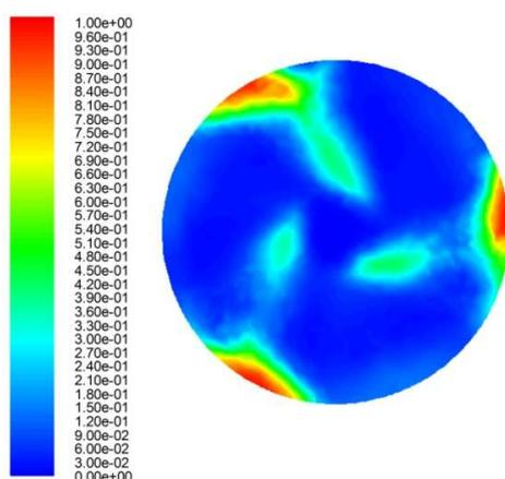
Figure 4. The contour of  $\text{CH}_2\text{Cl}_2$  volume fraction at cross section A-A of MIJSN
