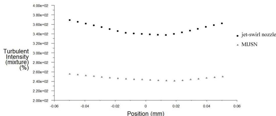
Figure 12. The distribution of turbulent intensity on the diameters of outlet for MIJSN and jet-swirl nozzle
