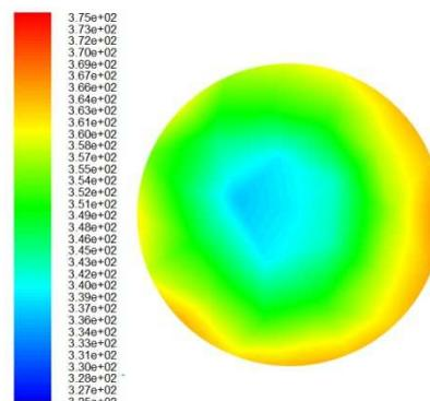
Figure 11. The contour of turbulent intensity in jet-swirl nozzle
