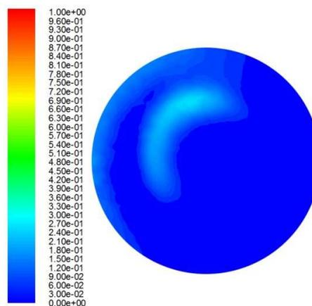
Figure 7. The contour of CH<sub>2</sub>Cl<sub>2</sub> volume fraction at cross section B-B of jet-swirl nozzle
