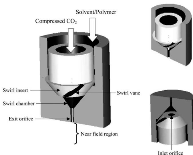
Figure 1. Schematic that illustrates the structure of the jet-swirl nozzle [13]
