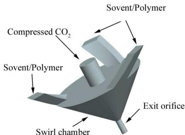
Figure 2. 3D geometrical computational domain of multi-inlet jet-swirl nozzle
